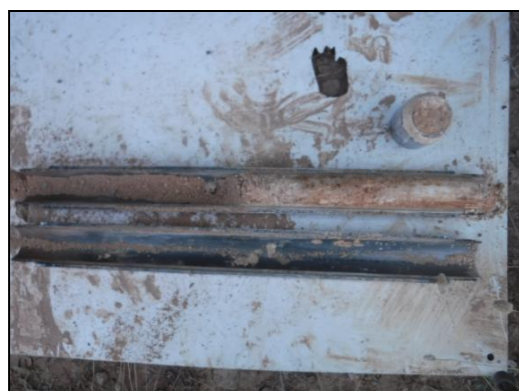
Foto 3: Sondeig S-1, SPT a 3,0 metres.
