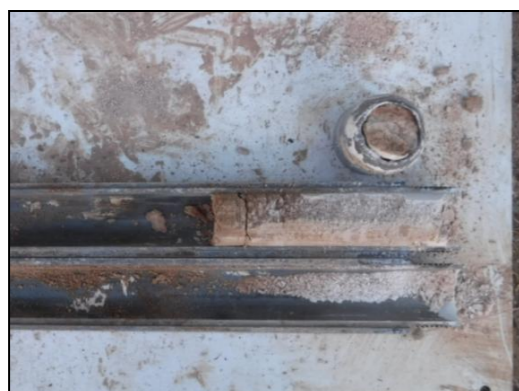
Foto 5: Sondeig S-3, SPT a 7,0 metres.
